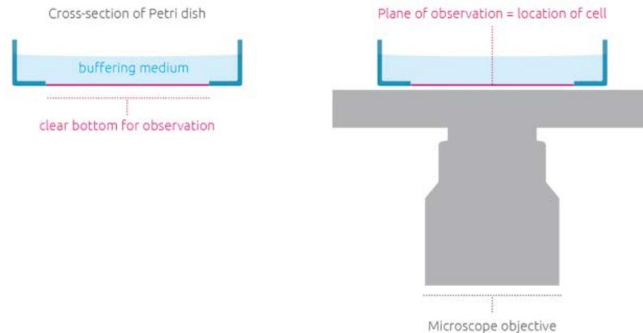
Figure 4. Schematic of observation of cells with the 3D Cell Explorer located in dish with glass bottom surface.
