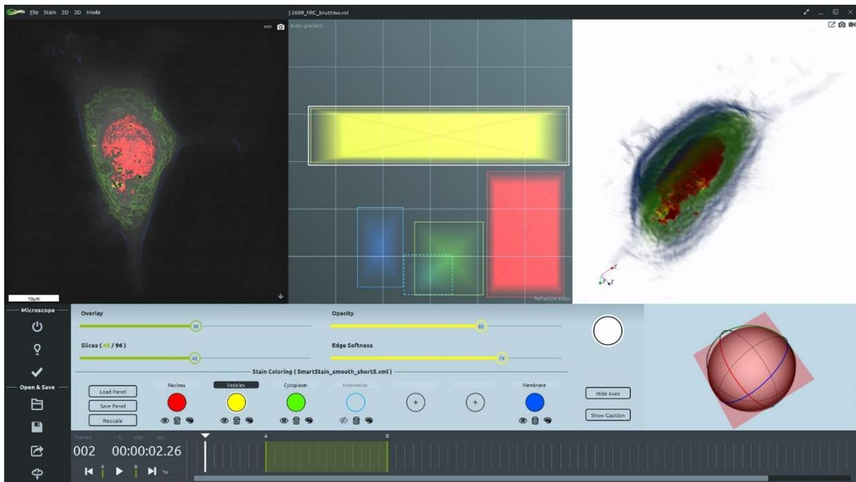
To mark and label certain parts of the measured cells in 3D, the software allows the user to “virtual brush” and digitally “paint” the part of a cell based on their physical properties (called refractive index). STEVE will automatically define all regions with same refractive index characteristics (different organelles have different optical properties) and digitally stain them with the same color. This process is quantitative and can be applied for a limitless amount of
